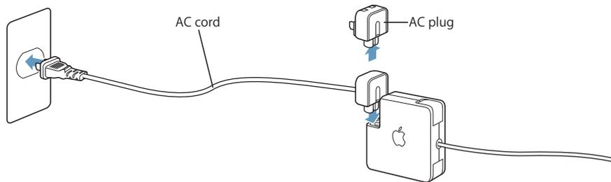
**Warning:** Make sure the power adapter is fully assembled before plugging it into an electrical outlet. If you're using the AC plug with your power adapter, make sure the two prongs are snapped into their completely extended position before plugging in the adapter.
