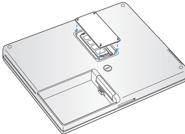
**Note:** To avoid damage, be careful not to overtighten the screws.
