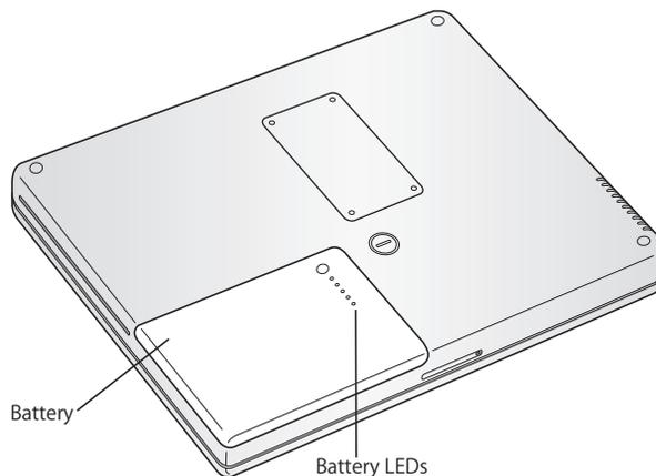
If the battery icon in the Finder menu bar is set to show the percentage of charge, you may sometimes notice that the battery does not maintain a full charge of 100% when the power adapter is attached. When the battery level eventually drops below 95 percent, it will charge all the way to 100 percent. This saves battery life as charging is not continuously cycled on and off.
