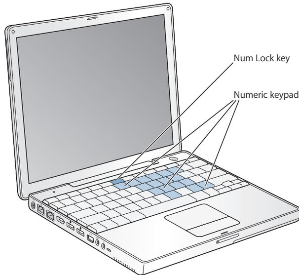
To use the numeric keypad, press the Num Lock key. The Num Lock key glows green, indicating that the keypad is active. When you're finished, press the Num Lock key again to turn it off.
